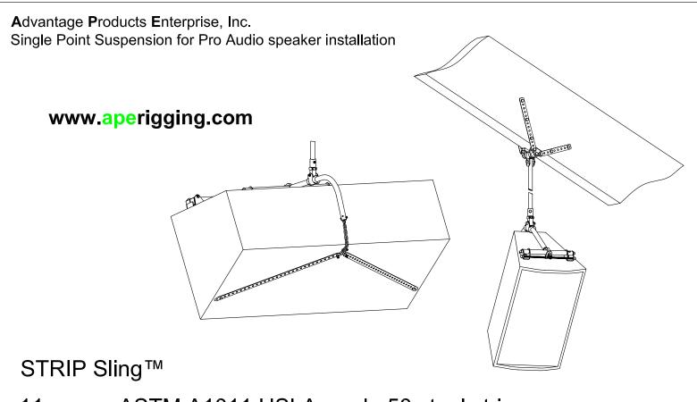
11 gauge ASTM A1011 HSLA grade 50 steel strips for low profile bridles and miscellaneous load securement
